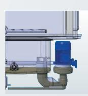
Self-draining wash pumps provide maximum hygiene with no smells and all wash and rinse zones drain automatically at the push of a button.
