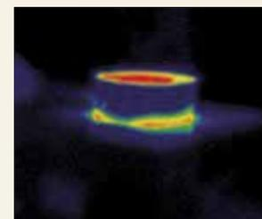
Heat radiated from induction hot plate (Efficiency 90%)
