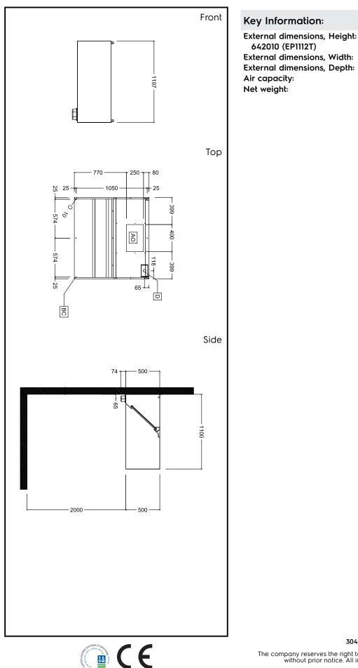
Ventilation Equipment 304 S/S Wall Hood+Filters 1200X1100mm
